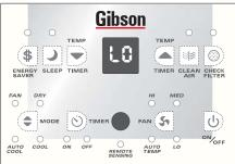
In the fan mode if "LO" or "HI" is displayed, this means the room temperature is outside the unit set points of 99°F/37°C (HI) or 32°F/0°C (LO).
